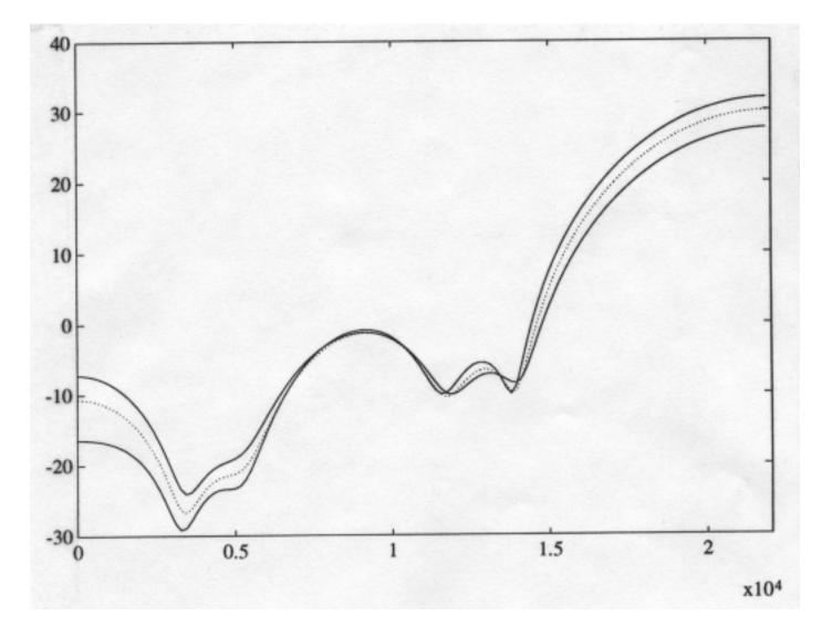
Figure 4: A set of three plausible curves for the frequency response of a noise-shaping filter. There is no absolute way of deciding which one of these curves is "best." The decision must be a subjective one.
