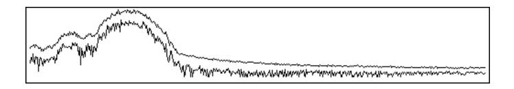
Figure 11: Spectrum of a signal with noise-shaped dither that has had varispeed (sample-rate conversion) applied. Note that the high-frequency energy of the spectral shaping is now shifted down to a region of the spectrum that is highly audible (the scale is linear, 0 to 24000 Hz).
