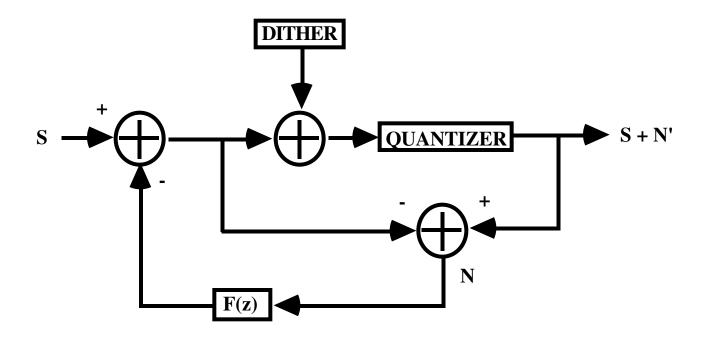
Figure 1: General block diagram of noise-shaped dithering. For unshaped dither, F(z) would be zero. For undithered noise shaping, the dither would be zero.
