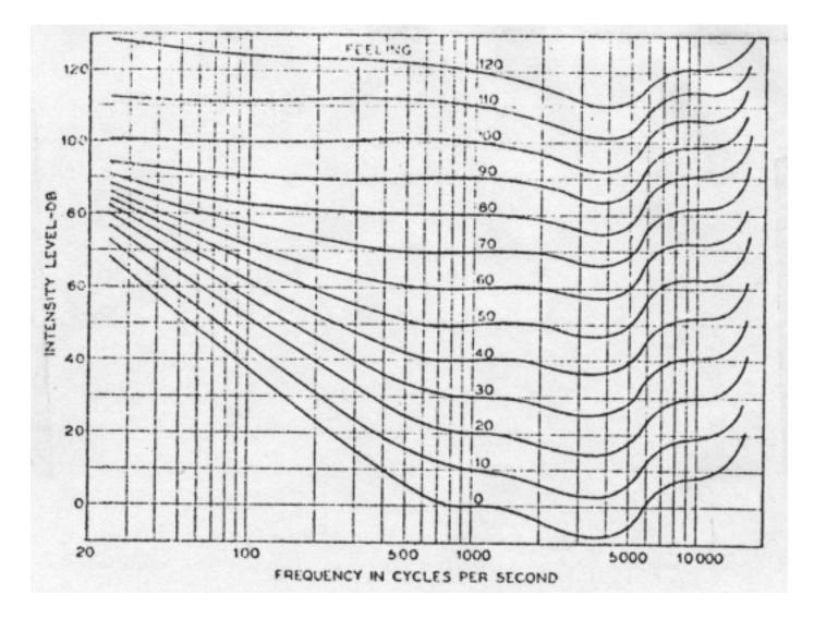
Figure 2: The equal-loudness curves reproduced directly from the 1933 article of Fletcher and Munson [5]. The signal used for these measurements were presented from a single loudspeaker placed directly in front of the subject.
